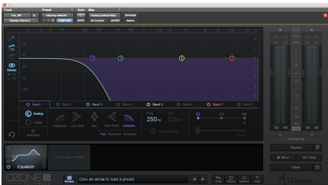
Figure 3.4.4: LPF at 250Hz for the Fukada LL and RR Channels
