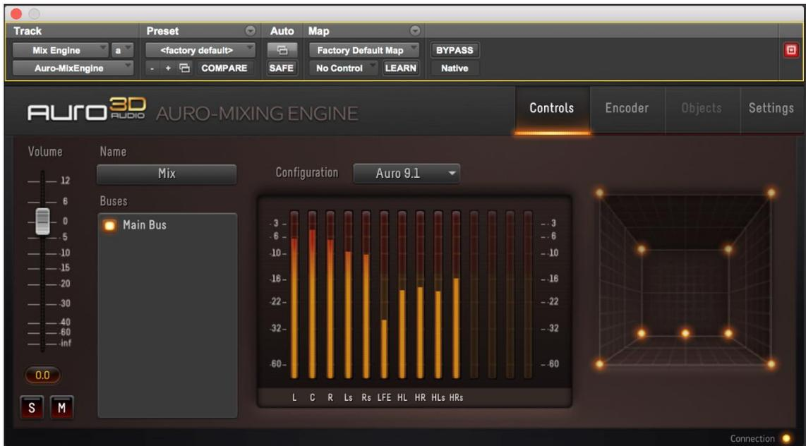
Figure 3.4.7: Auro-3D Mixing Engine Displaying the 9.1 Mix
