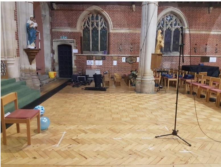
Figure 9.7.1: Impulse Response Recording of Balloons on the Position of the Front Arrays
